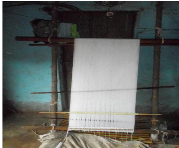
Plate 2: Frame loom previously used to weave Akwa Ocha in South-south Nigeria (Own image)
